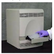
3. Load the 96-well optical plate with the notched A12 position at the top-right of the tray.
