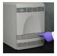
2. Load the plate into the plate holder in the instrument. Ensure that the plate is correctly aligned in the holder.
