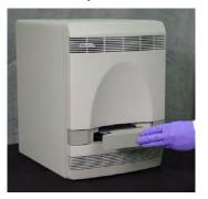
5. Apply pressure to the right side of the tray and at an angle to close the tray door.
